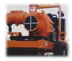
DriveDiesel driven.FlowFrom 30m³/ hour to 3000m³/hour.HeadFrom 10m to 250mVacuum Assist Diaphragm, Compressor and Rotary Valve.
